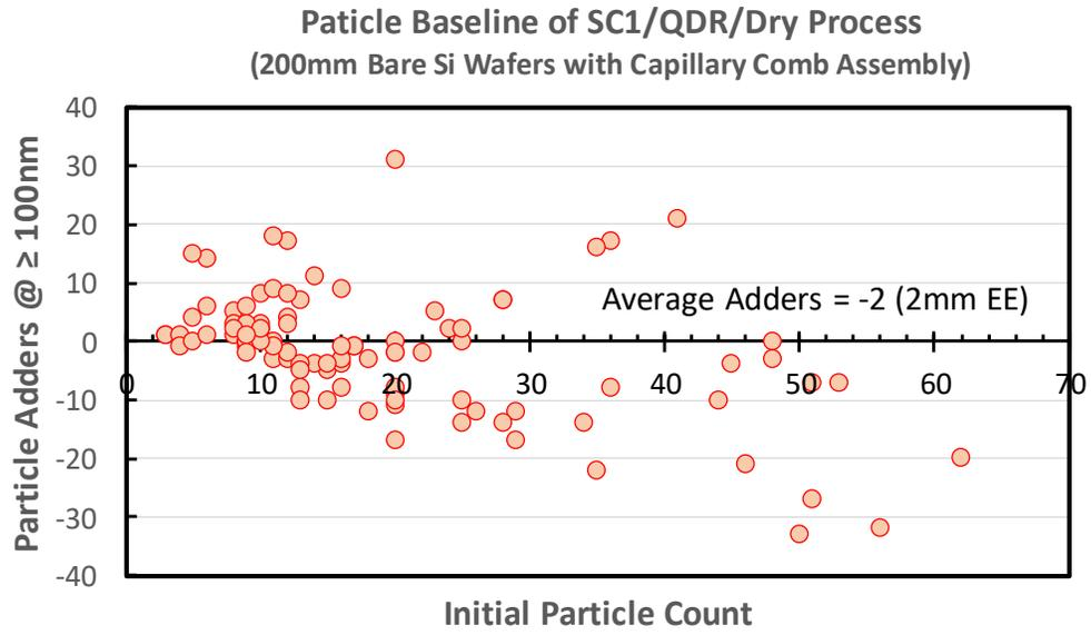
Figure 6. Particle performance of a Marangoni dryer using a capillary comb assembly.
