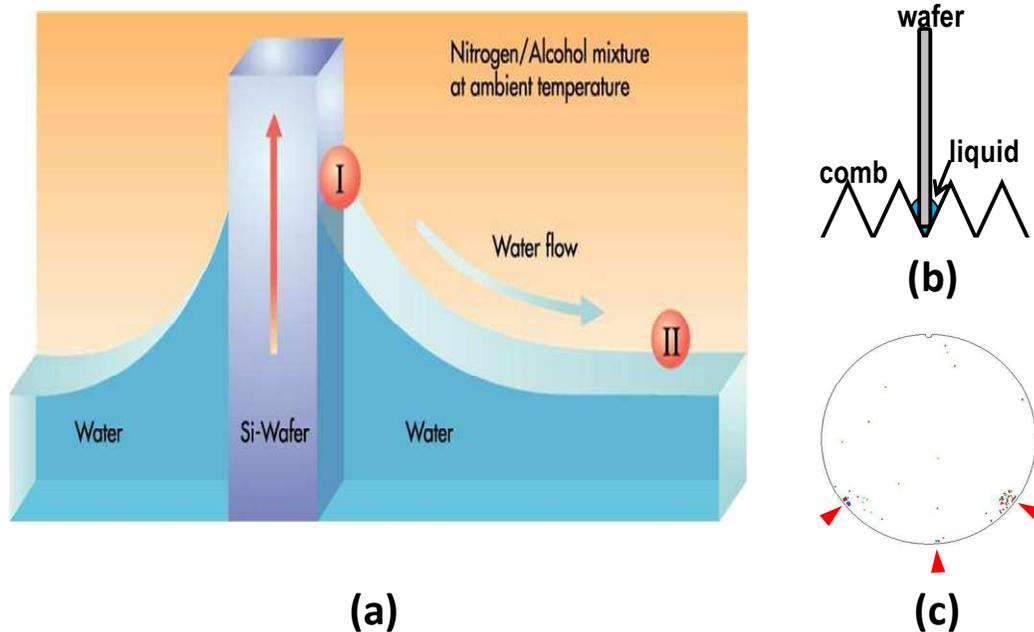
Figure 1. Marangoni wafer drying process is schematically illustrated in (a), likely inducing wafer contact mark contamination which is related to liquid retention at the wafer/holder contact area (b) and revealed by a wafer particle map (c).
