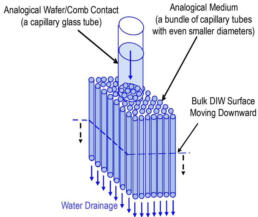
Figure 3. Conceptual modeling of a technical approach for eliminating water retention at the wafer/holder contact area.
