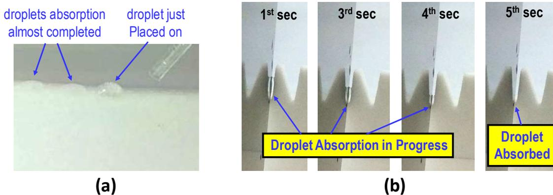
Figure 4. Water droplet absorption testing is performed on a capillary medium with a strip sample in edge-on position (a), and a Si wafer at the wafer/comb contact (b).
