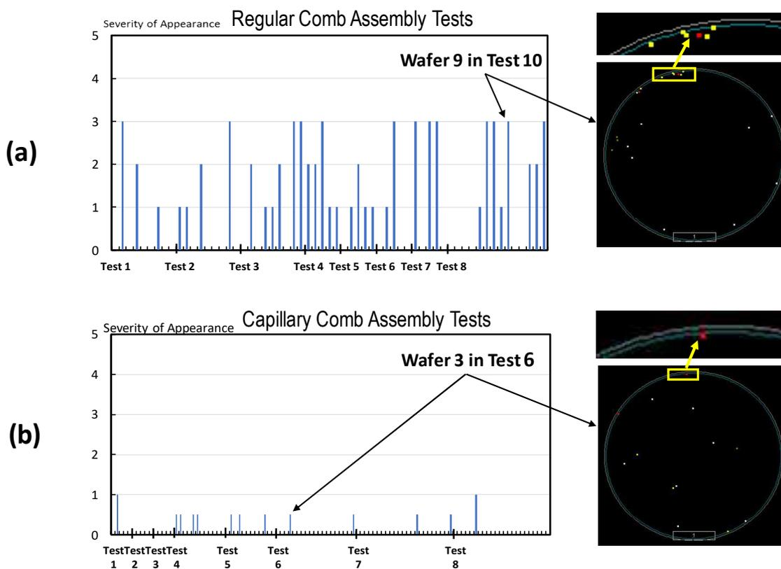
Figure 5. Comparison of contact mark incidence between the use of a regular comb assembly (a) and a capillary comb assembly (b) in a LuCID™ dryer. The severity of appearance (Y axis) is rated against particle number in a contact mark; i.e. 0.5 (one particle), 1 (two particles), 2 (3-5 particles), 3 (> 5 particles).
