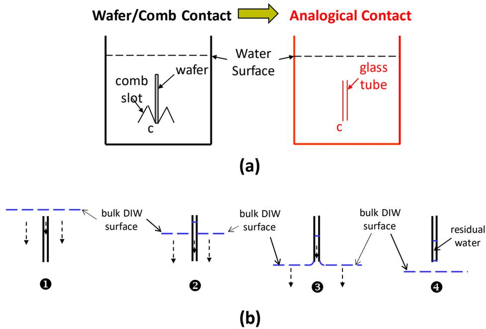
Figure 2. Schematic illustrations are used to interpret the analogy of a wafer/holder contact area (a), and how water retention at a contact area occurs in Marangoni drying (b).
